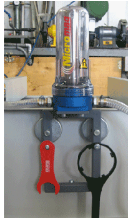
Figure 1A Micromag filter installed. It's the basic model magnetic filtration system available in three sizes (5, 10, and 20 inches) from Eclipse Magnetics, for filtering ferrous particles from machine coolants and lubricants at flow rates up to 150 liters/minute
