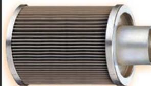
These are BIG suction strainers. They thread onto reservoir suction pipes inside the tank. They are available as large as 8" diameter, up to 6" npt, and can handle flow rates up to 600 gpm. Both male and female pipe connections are offered. Stainless steel wire cloth is standard with mesh sizes of 30, 60, 100, or 200. Each flow rate is offered in more than one length/size configuration to fit your available space. Give us a call for more information.
