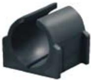
**THE CUSHION** Manufactured from a thermoplastic elastomer. It’s built tough to withstand the effects of most oils, chemicals, and other industrial fluids, in temperatures from -50°F to 275°F. Interlock edge insures the cushion remains in place.
